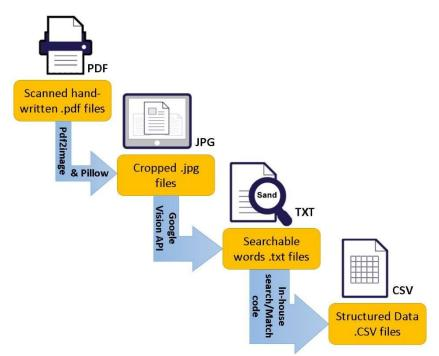
Figure 4. Flowchart of the proposed procedure to convert the handwritten data to .csv files.
