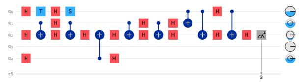
Figure1. Schematic of the quantum circuit implemented for quantum cheque generation on the IBM Quantum Experience platform.
